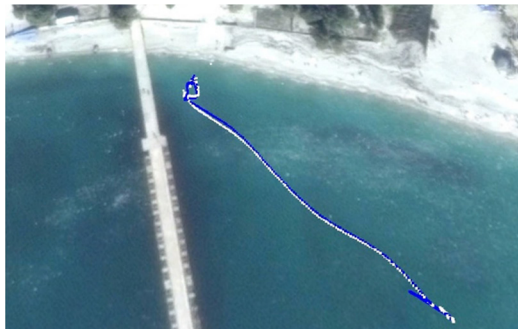
Fig. 10. The AUV's trajectories calculated by reference and designed systems (AUV prototype field testing with reference system installed)
